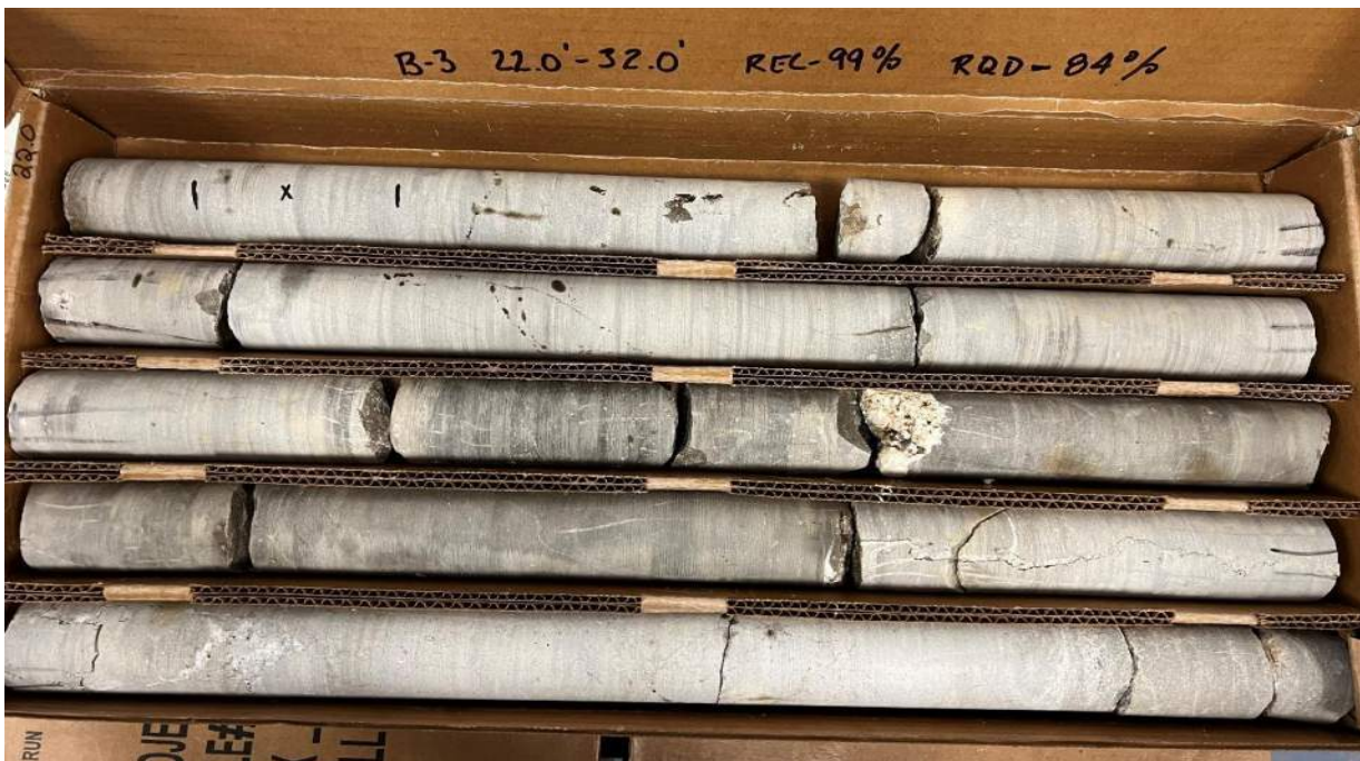
PHOTOGRAPH 16 - B-3 ROCK CORE (22.0' - 32.0')
