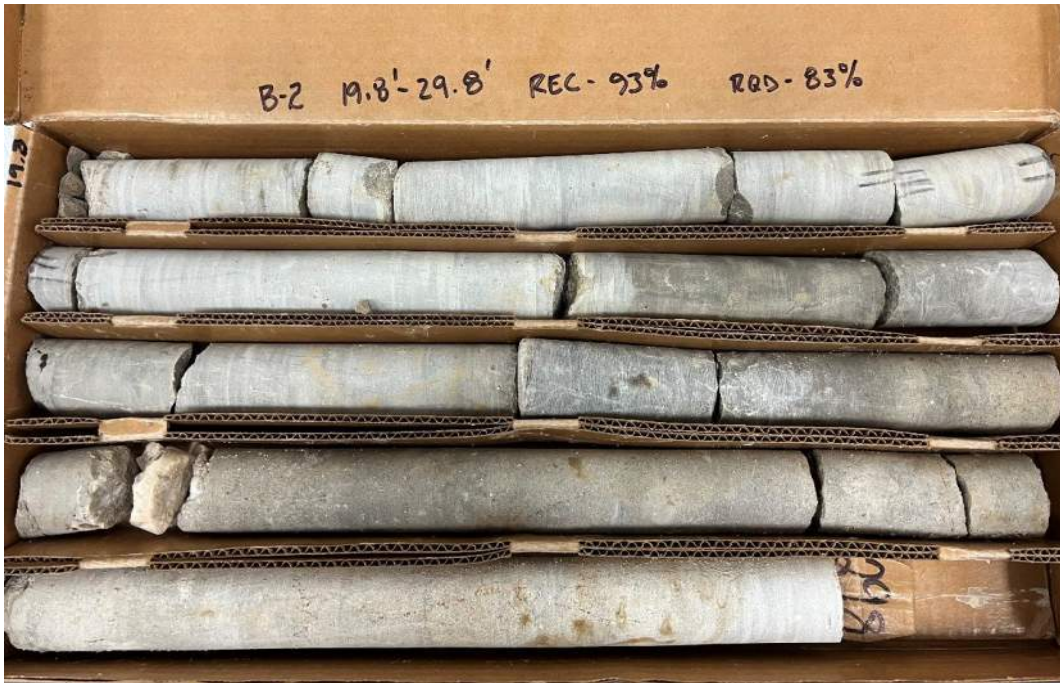
PHOTOGRAPH 14 - B-2 ROCK CORE (19.8' - 29.8')
