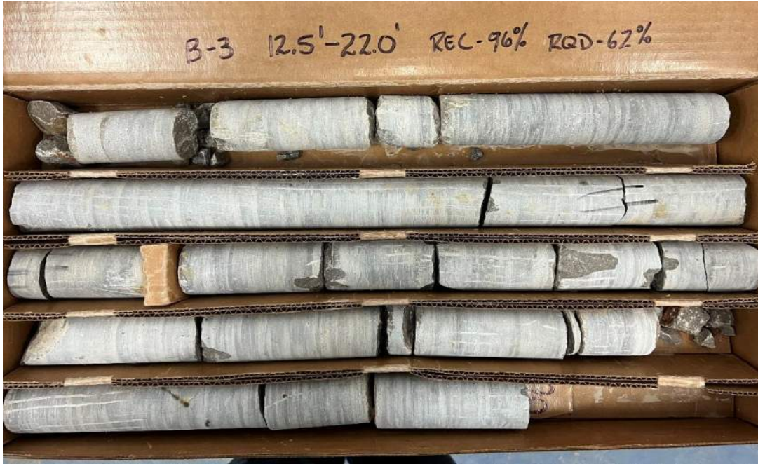
PHOTOGRAPH 15 - B-3 ROCK CORE (12.5' - 22.0')
