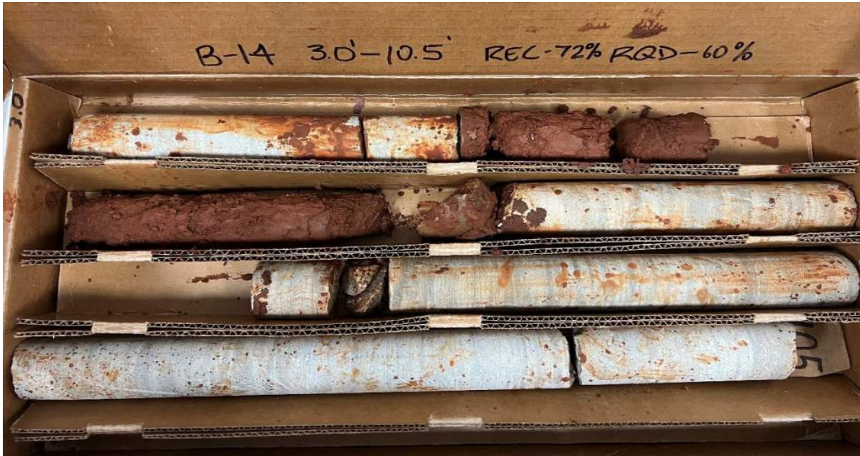
PHOTOGRAPH 17 - B-4 ROCK CORE (3.0' - 10.5')
