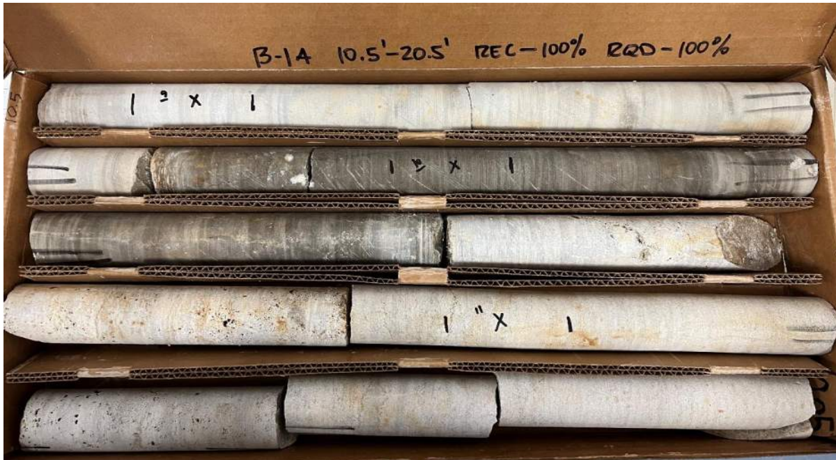
PHOTOGRAPH 18 - B-4 ROCK CORE (10.5' - 20.5')
